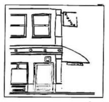
(iii) "Awning sign" means a structure made of fabric or similar material with a painted metal frame which is attached to a building and projects over a public walkway. An awning shall have no soffits, plastic components or internal lighting. Plastic awning fabrics are prohibited. Advertising material attached to an awning is an awning sign.
