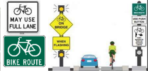
"Bikes on Bridge" activated warning.
