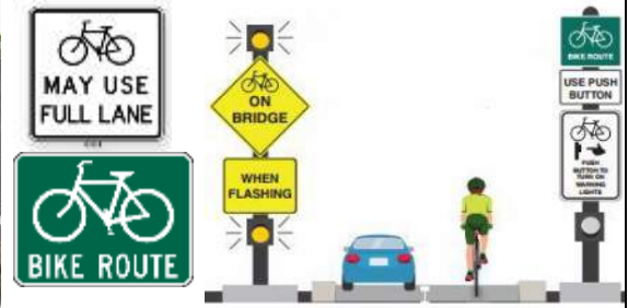
"Bikes on Bridge" activated warning.
