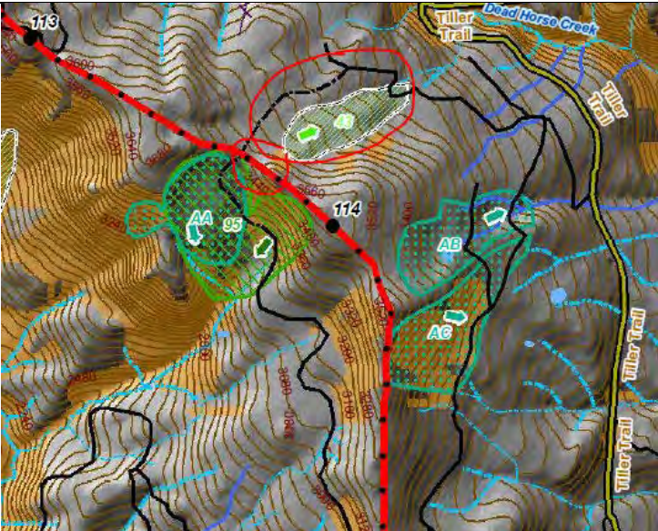
Location of PAR-113.66 and Proposed Road Reconstruction relative to landslide features. Figure 25 of 47. Note: the light brown areas are Potential Rapidly Moving Landslide Hazard
