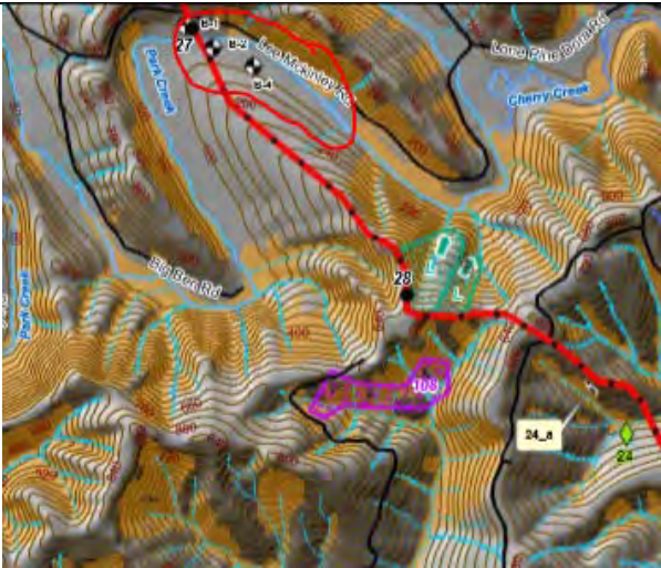
Location of TAR 27.06 near Milepost 27 on the Geologic Hazards Maps. Figure 8 of 47. Note: the light brown areas are Potential Rapidly Moving Landslide Hazard
