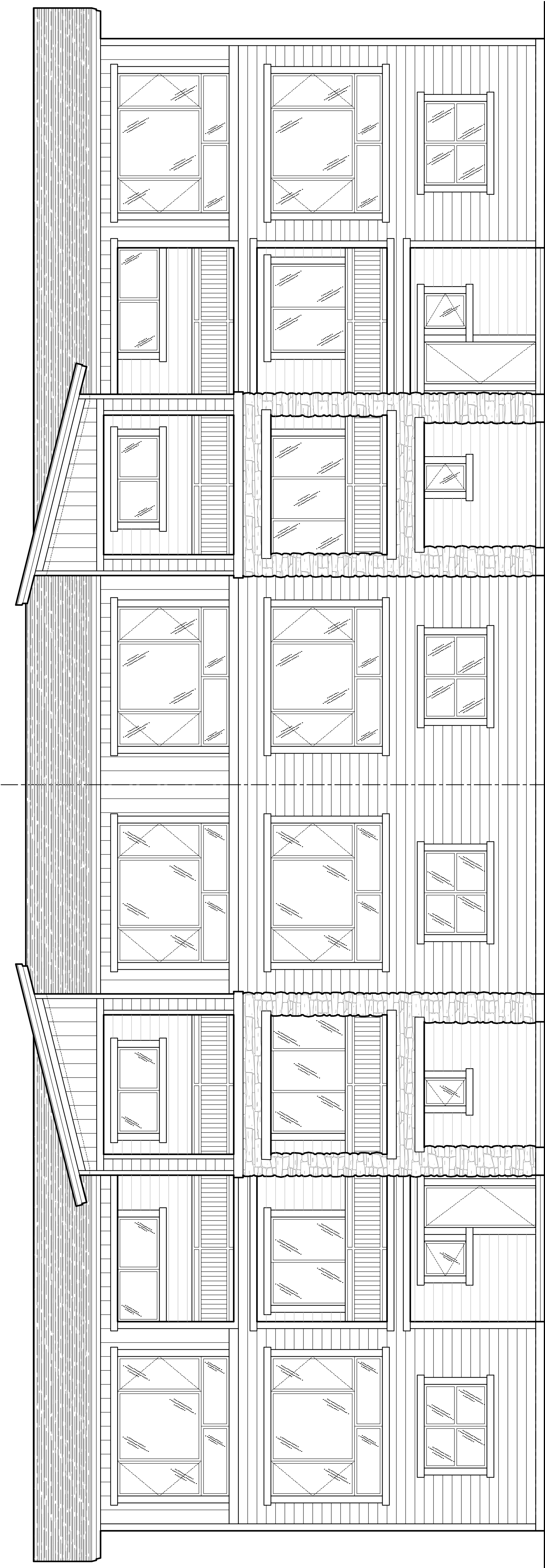
REAR ELEVATION - BAYSIDE UNITS BUILDING No.1 SCALE: 1/4" = 1'-0"
